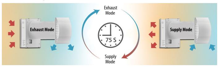
When two synchronized ventilators are operating in regeneration mode, one ventilator supplies air while the other ventilator exhausts air. In any other mode, the synchronized ventilators will operate in the same direction.
