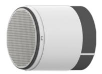
The high-tech ceramic energy regenerator provides a regeneration efficiency of up to 97%. The recovered heat from the exhaust air will heat or cool the supply airflow. Due to its cellular structure, the unique regenerator has a large air contact surface and high heat conducting and accumulating properties.
