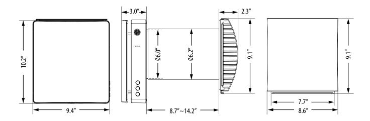
ECO-FLO*Plus* is suitable for wall thickness ranging from 8.7" to 14.2". Consult factory for walls thicker or thinner than the standard dimensions.
